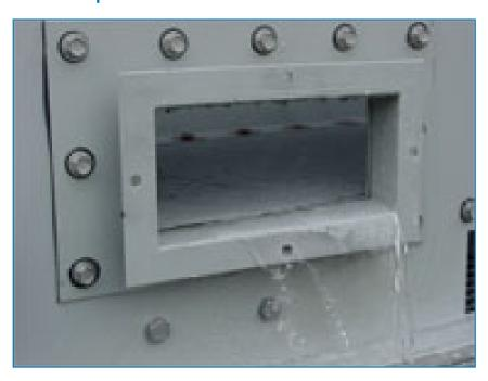
A factory-installed clean out port
