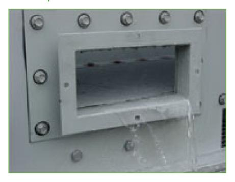
A factory-installed clean out port
