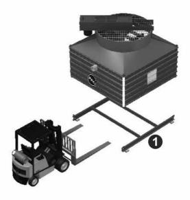
Figure 1: RCT Shipping Support for Casing Section
